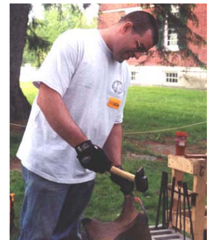
Andy VanSchoick forms an anvil 'hold-down' around and for the base of his anvil.
