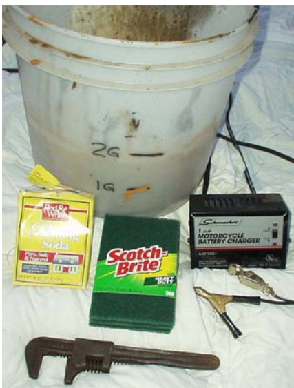
Everything you need for electrolytic rust removal. 5 Gallon bucket, baking soda, abrasive for making sure contacts are secure, battery charger, scrap metal (not shown) and a rusty item (monkey wrench)
