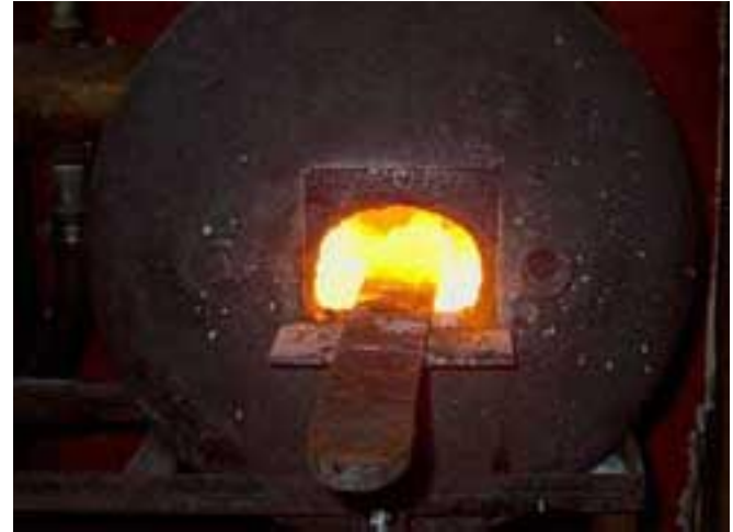
Figure 3 - End portion of the sword bar being heated to welding heat.
