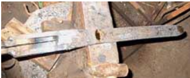
Figure 2 - Sword bar (2 core bars and a wrapped edge bar) welded two-thirds
