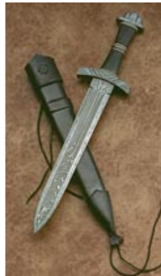
Figure 7 - Completed dagger made from the billet remain of another sword. Note the seam in the tip is nearly invisible.
