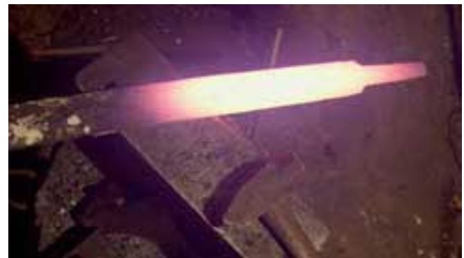
Figure 4 - Sword bar completely welded. Note the even color indicating all source bars are fused into a solid mass.
