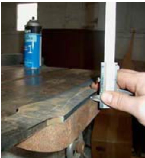
Figure 1 - Scribing the center line of the edges. The line then becomes a target to grind to.
