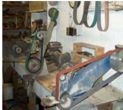
Figure 2 - Mr. Cashen's grinders. Both are wired in such a manner that the air handling system for the shop must be on in order for them to work. This helps keep grind particulate to a minimum
