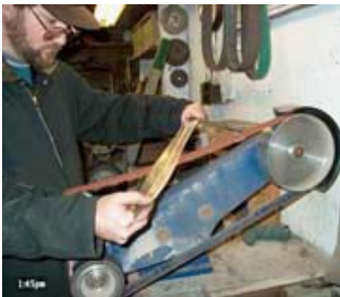
Figure 8 - Working with a 'slack belt' assists the transition from edge to blade face.
