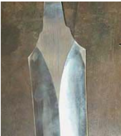
Figure 4 - The complex sweeping curves near the ricasso needed to be 'sculpted' by hand with files and stones.
