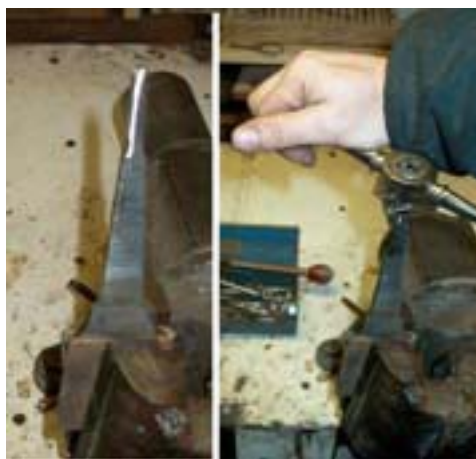
Figure 9 - With the edge and other blade sections ground to within .025" the tang is threaded to a receive the pommel. This will enable further and even more precise weighing.
