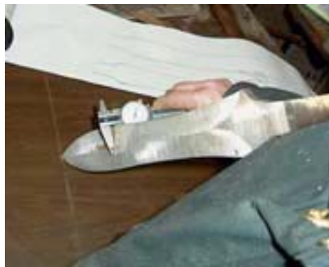
Figure 5 - Checking the distal taper (the rate of thinning from ricasso to tip) with a micrometer.
