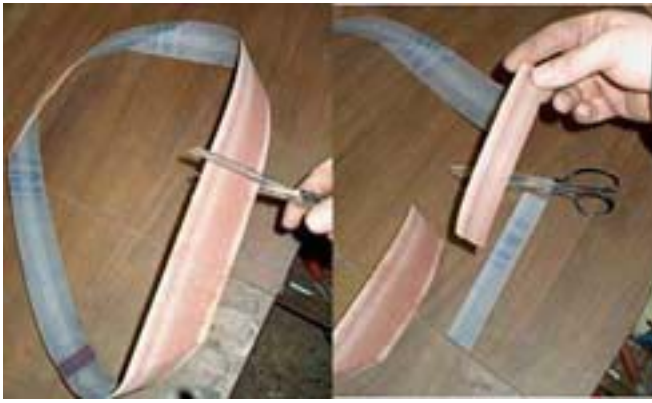
Reusing the belt grinder belts for the polishing sticks.
