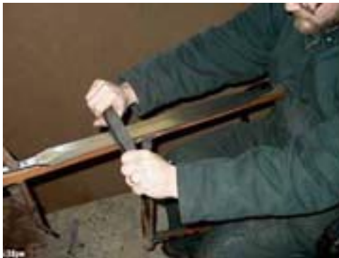
Polishing chair in use with the polishing stick. Working by hand 90deg from the machine grind yields clear results.
