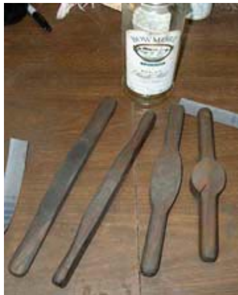
Various wooden polishing blocks. With sandpaper attached these wooden polishing closely form to the curves of a blade.
