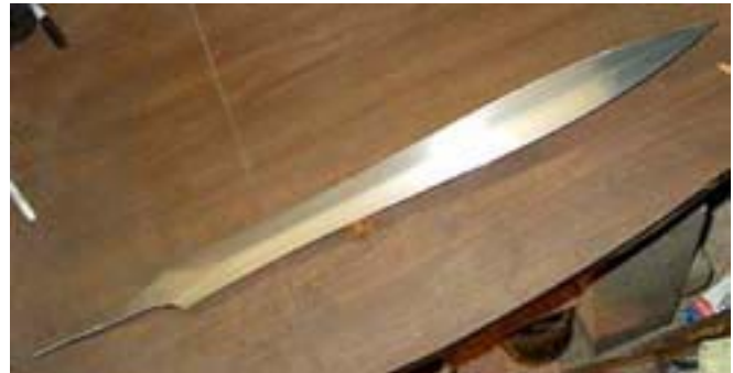
Completely polished blade waiting for final heat treatment.
