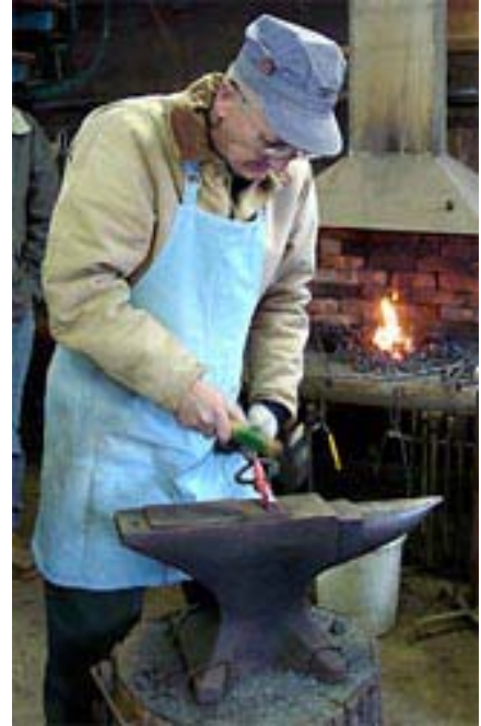
Jim Moran hammers an edge onto a cold chisel. Photo by Thom Breitenbach.
