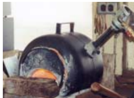
Home made propane forge built by Andy VanSchoick from an old propane tank.
