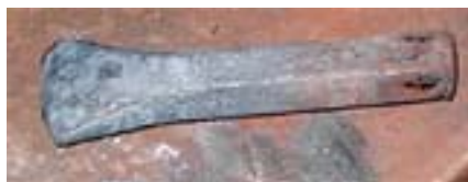
Figure 2 - Rough shape, note the slightly curved cutting edge.
