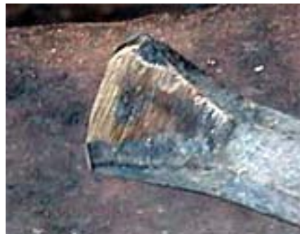
Figure 3 - This chisel shows the range of temper colors; light yellows right down to blues, and purples (Figure 3)
