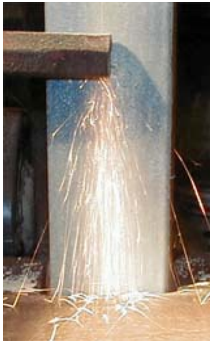
Figure 1 - Bright sparks indicate this is a relatively high carbon steel
