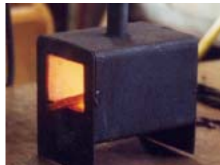
Home made propane forge built by Doug DeLurey using 1/8” box tubing and home made
